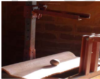
REPRESENT 7: view of the trial device of shock resistance
